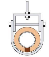
**Recommended Installation Instructions** GLT Wood Blocks are placed inside the pipe insulation at the hanger location. Before applying the pipe insulation simply notch out the insulation with a knife and replace it with the appropriate size wood block (see sizing chart). Proceed by applying the pipe insulation to the pipe and then inserting the appropriate GLT Saddle.
