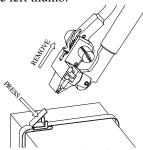
10. Hammer down wings securely using hammer knob on tensioner, or a similar tool.
