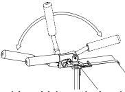
7. With strap tightened, bring tension lever back to original position, hold both handles together, and tilt forward as shown.
