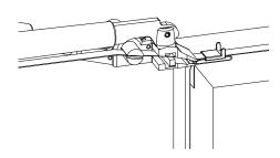
6. Holding the shear lever with the right hand, push the tension lever back and forth in a full arc with the left hand to tighten the strap.
